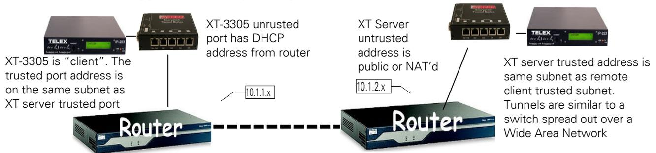
Telex IP addresses: 192.168.2.x at both ends of the link.
